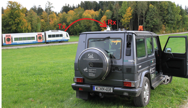
Fig. 2. T2T measurement setup: Rx on the car in the foreground and Tx on the train in the background
