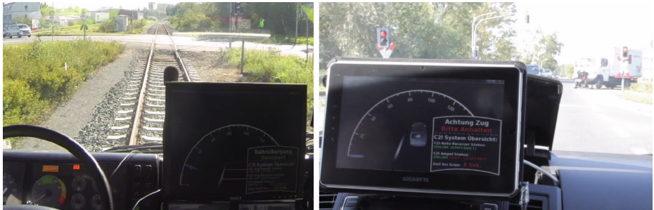
Fig. 2. User Interface in the train (left) and car (right) at Demo Situation with LX activated.
