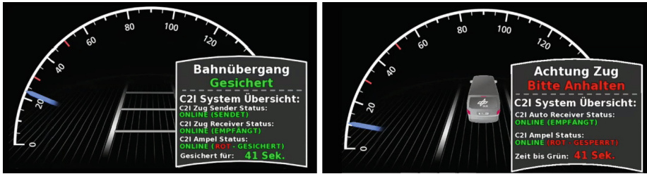
Fig. 3. User Interface design in the train (left) and the car (right) at Demo Situation with LX activated
