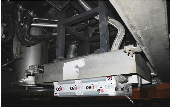
Fig. 2. BTM test antenna installed under a train
