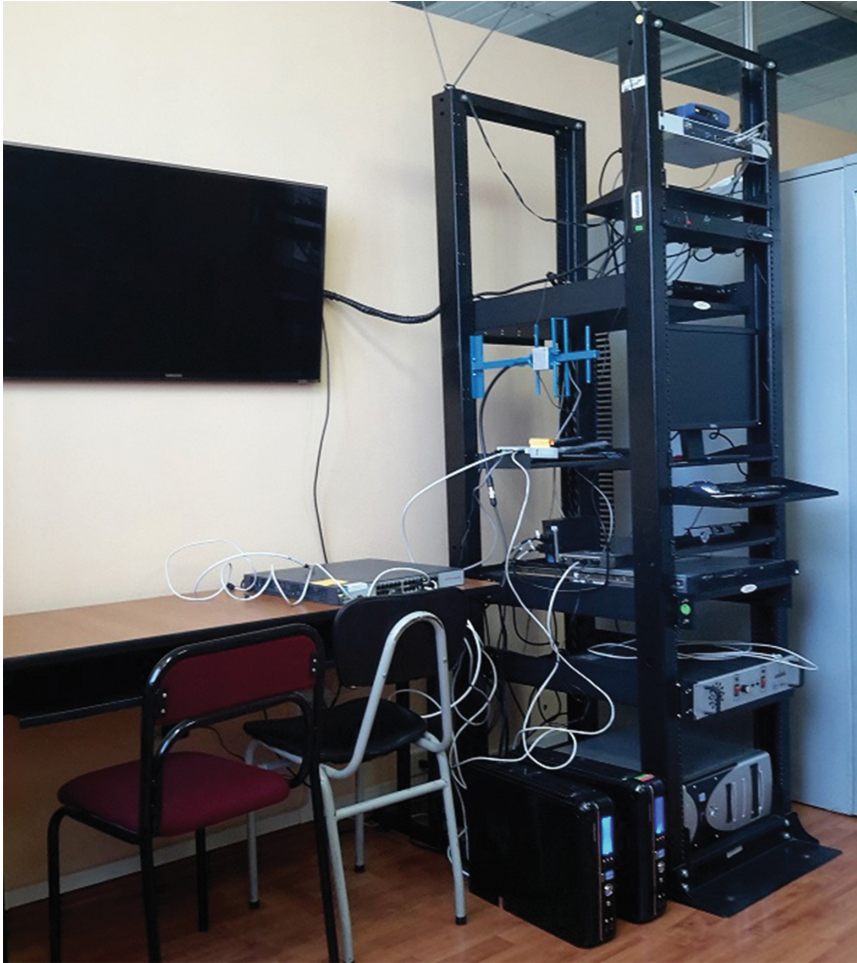
Fig. 5. EiTv playout generator, Telavo amplifier and Yagi antenna
