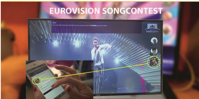
Fig. 2. On the second screen app or from the TV-show the question appears that must be answered. On TV’s HbbTV layer the answer of each player is displayed, using signaling colors such as green (good answer) and red (wrong answer) – example from “Eurosong”. (Color figure online)
