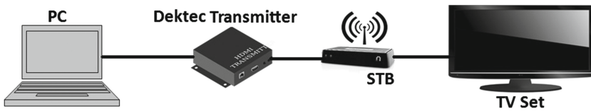
Fig. 4. Scenario for testing the generated BTS.
