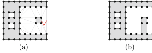
Fig. 7. Solving the instance from Fig. 4 with a tail cut (red line). (a) The red curve needs to be crossed at least twice or two edges must leave the component. The red curve is found via the Delaunay Triangulation (grey). (b) The first iteration after using the tail cut. (Color figure online)
