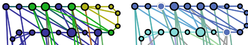
(a) Excerpt from a partition where the gap constraint is violated, since nodes 4 and 6 (counting clockwise from the upper left) are in the green fragment, but node 5 is in the blue fragment.
