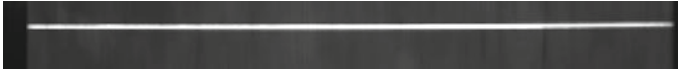
Fig. 14 Picture which has been through image mosaicking and extracted the area with only laser line on
