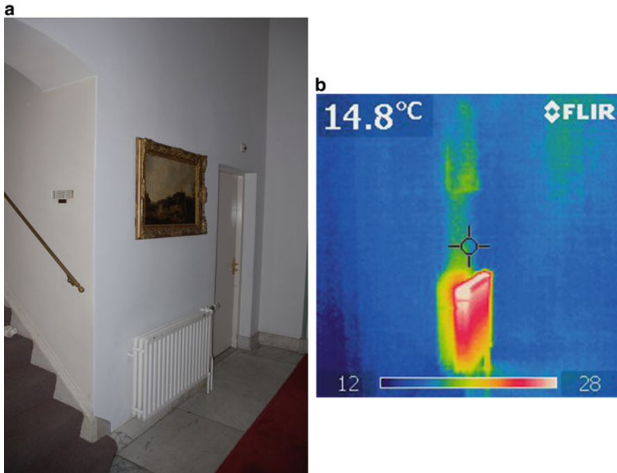
Fig. 7.11 A painting hanging over a radiator, with a low temperature set point (a). In the thermal image (b) a subtle heating of the underside of the canvas painting can be clearly seen
