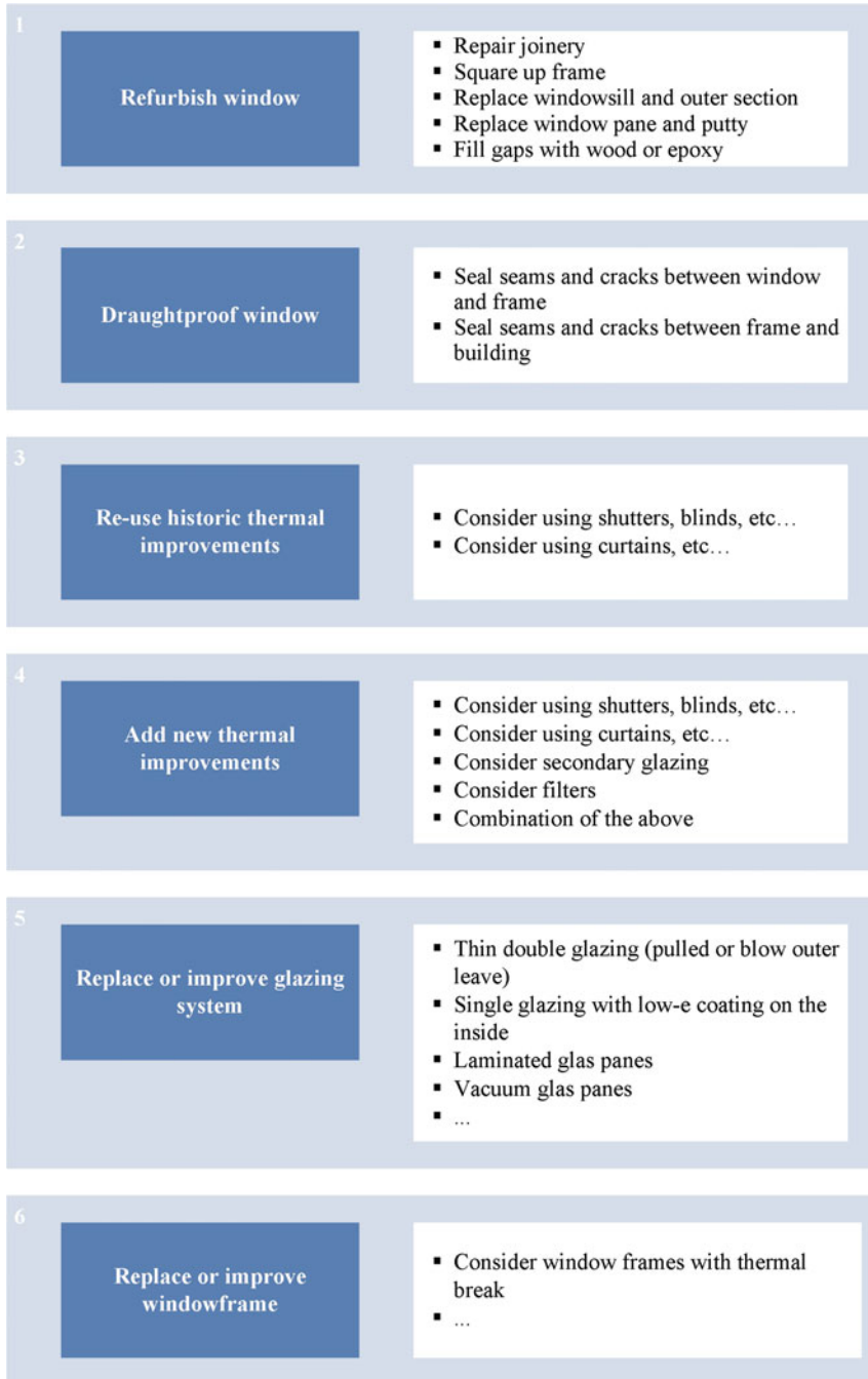
Fig. 9.4 Six steps to optimize a window to reduce the impact on the indoor climate
