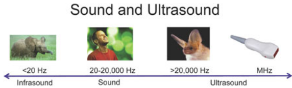
Fig. 3.3 Sound frequencies. Medical ultrasound is in the Mega-Hz (million Hz) range
