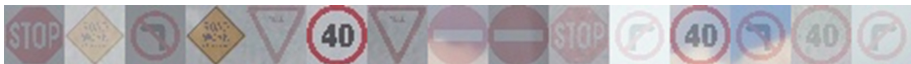
Fig. 2. Sample of testing set traffic sign images ( 32 \times 32 pixels) with fog filter opacity in range 50–90 %
