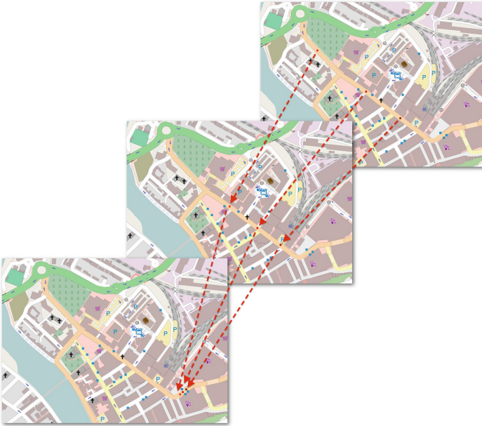
Fig. 21. Because of delays caused by boarding passengers the headway between buses is successively eroded over time until the buses are essentially ‘clumped’ together. (Color figure online)
