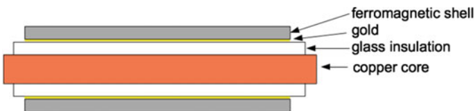
Fig. 6 Bi-phase wire with glass insulation between copper core and ferromagnetic shell
