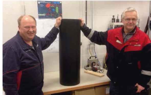
Figure 16 The fuel grain for the Unitary Motor
