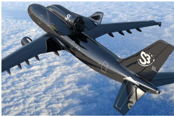
Figure 10. An artistic image of the SOAR system during a flight of the carrier airplane.
