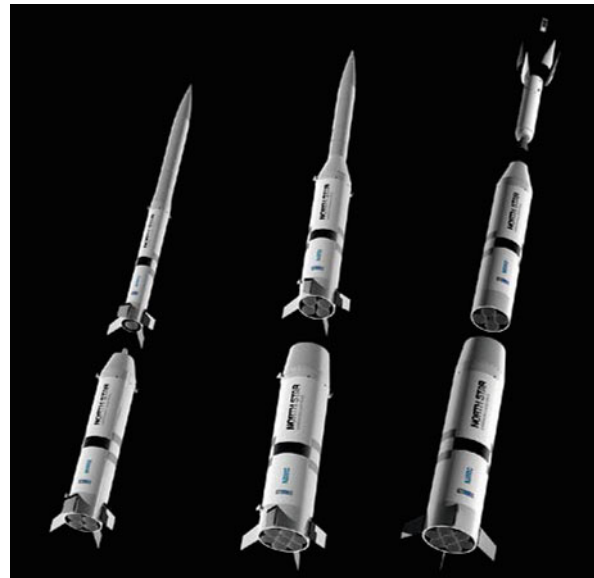
Figure 9 A modular concept is adopted and engines and complete stages are reused (Source: ASC)
