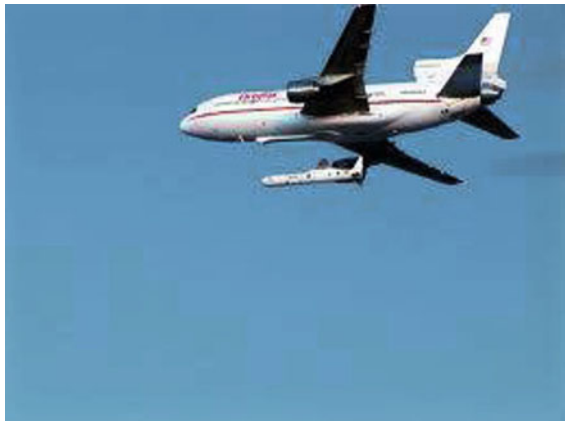
Figure 1. The ‘Pegasus’ system that is the only operational example of the air launch concept but is not featured with a high economic efficiency
