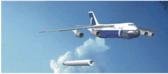
Figure 5. An artistic image of the 'Air Launch' system in flight at the moment of launch vehicle ejection
