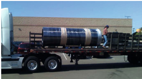
Figure 6. Local Transport of a 200-cuft., 500-psi LOX Tank.
