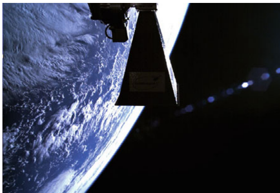
Figure 3 – ‘Selfie’ of SSTL high gain antenna pointing mechanism on board TechDemoSat-1
