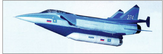
Figure 11. A model of the 'Ishim' launch system – the MiG-31I carrier aircraft with a suspended launch vehicle
