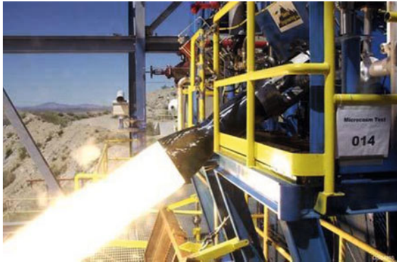
Figure 11. 20K lbf Thrust Engine Firing Test (Edwards Air Force Base).
