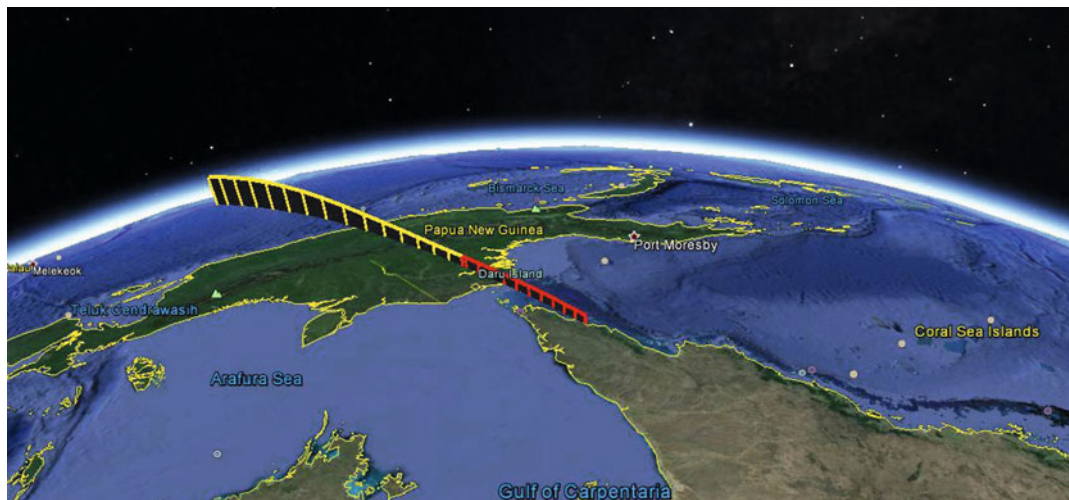
Figure 6. Launch trajectory from Cape York Australia. SPARTAN flight shown in red and 3 rd stage trajectory shown in yellow.
