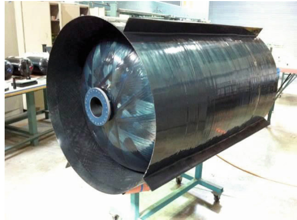
Figure 5. All-Composite Tank with Skirts and Longitudinal Stringers.
