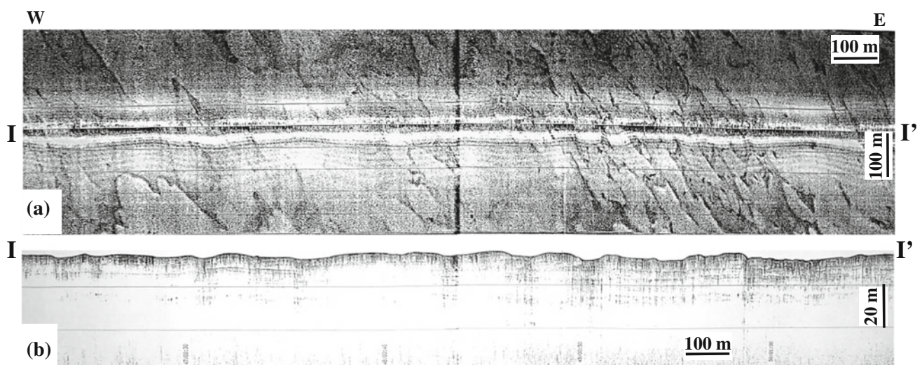
Fig. 43.4 MAK I sonograph (a) and 5-kHz seismic profile (b) along lines I-I' of the southwestern sector of the channelled-unchannelled transition zone on the Valencia Fan, showing bands of ellipsoidal patches believed to be megafaults
