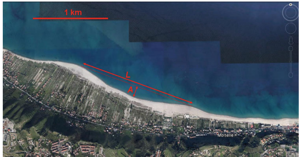
Fig. 11.1 km-scale shoreline sand waves near Mortelle (NE Sicily). Definition of the wavelength, L , and the amplitude, A . Source Google Earth, image from 2016 TerraMetrics, map data from SIO, NOAA, US Navy, NGA, GEBCO
