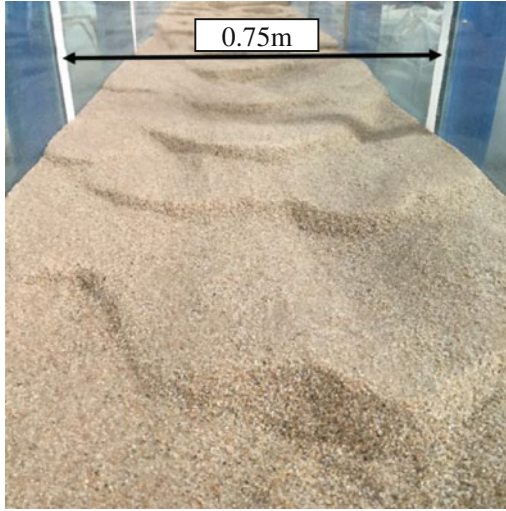
Fig. 3.1 Dune field generated by a current in the laboratory. Experiment performed at the Hydraulics Laboratory of the UCLM
