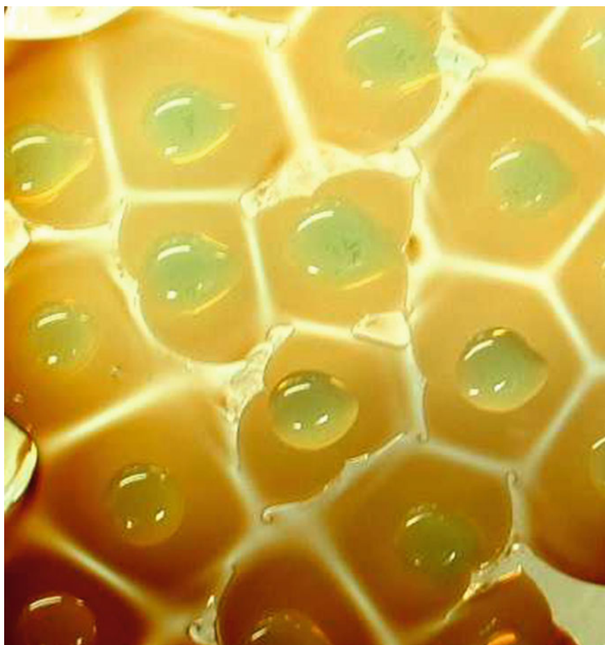
Fig. 7.14 Failure to compute Voronoi diagram due to chemical instability which disrupts the circular fronts
