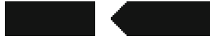
Fig. 5.2 A classical chemical signal diode [3]. Grid size is 120 \times 60 , the channels are 20 grid points wide and the gap is 8 grid points wide
