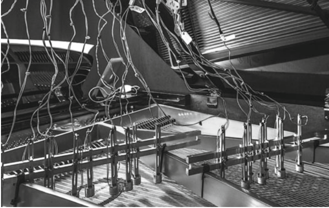
Fig. 29.15 The biocomputer plays the piano through electromagnets placed on the strings
