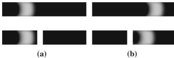
Fig. 5.3 Pulse delay by penetration property of the BZ reaction. Grid size is 120 \times 80 , the channels are 20 grid points wide and the gap is 8 grid points wide. It leads to 13-grid point delay after penetration. a Pulses propagation before penetration. b Pulses propagation after penetration
