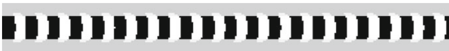
Fig. 6.5 Example time-lapse output from the simulator. The activator concentration is thresholded at u = 0.04 every 1000 simulated time-steps, and marked as white . The illuminated (passive) regions of reactor (high \phi ) are signified by grey background, and non-illuminated (active) regions of reactor (low \phi ) are black
