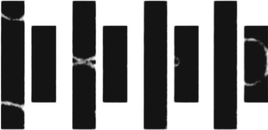
Fig. 6.2 Four photographs of a chemical coincidence detector. Each photo has two sections of active substrate, the left-most acting as inputs, the right-most as output. The waves are inputted (from the top and bottom ), and as they collide, the activator concentration between them rises higher than if only one wave was present. This results in the activator diffusing farther into the gap between input and output section, producing a wave on the output section (from [16])
