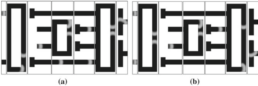
Fig. 5.17 Simulation results of two-bit binary adder when inputs ( A_1A_0 and B_1B_0 ) are a 10, 01. b 10, 11
