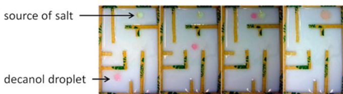
Fig. 11.1 Maze solving decanol droplet. (Supplementary movie in youtube http://youtu.be/P5uKRqJJeSs ). Reprinted with permission from [16]. ©2014, American Chemical Society
