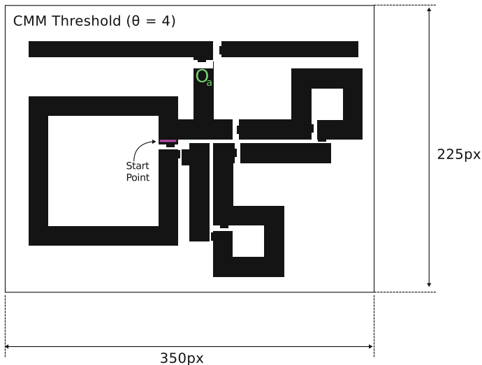
Fig. 6.14 Reaction layout for thresholding logic with threshold value \theta = 4 . The two memory cells on the right and bottom are the binary counter, and the large memory cell on the left produces the output waves to inhibit the output line (across the top )
