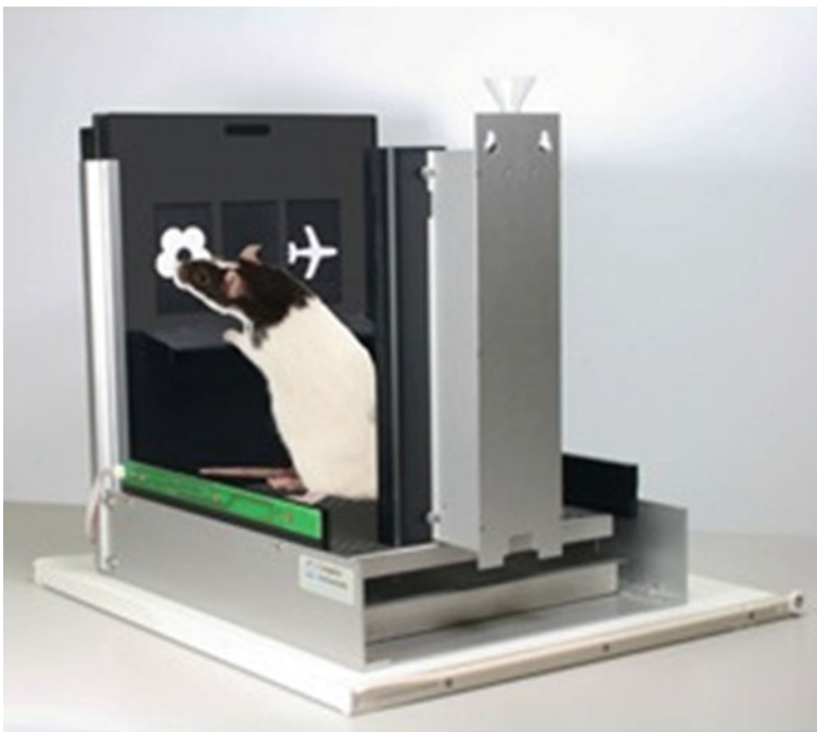
Fig. 1 The rodent touchscreen operant chamber allows for the flexible presentation of visual stimuli at any location on the screen (image courtesy of Campden Instruments). Screen masks are used to frame the response locations relevant to a particular task. Rats or mice respond directly to the stimuli by breaking the infrared beams overlaying the touchscreen with their nose. Appetitive reinforcers are delivered in a reward magazine to the rear of the chamber
