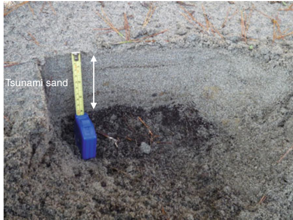
Fig. 3.10 11-cm-thick sand layer at 0.6 km from the shoreline (site b8 in Fig. 3.7b) in wide strand plain at Sendai City
