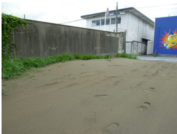
Photo 6.1 Liquefaction point at Sawara located in the former river course (taken in July 2011)
