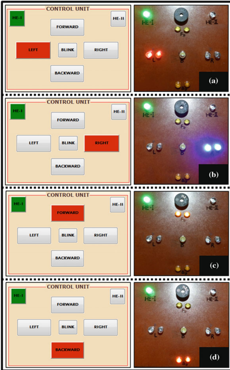
Fig. 13 Control task execution and hardware realization a left eye movement-left command b right eye movement-right command c up eye movement- forward command, and d down eye movement- backward command
