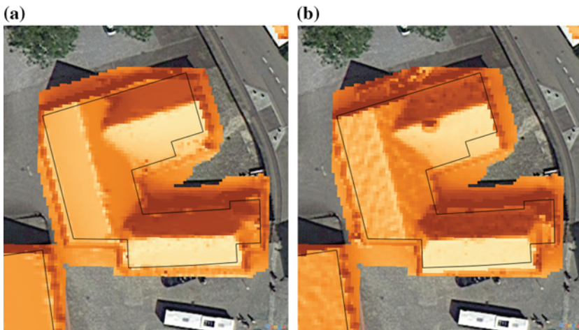
Fig. 8 Comparison of solar radiation estimates using the same method with the new DSM as well as reference DSM. a New DSM. b Reference DSM
