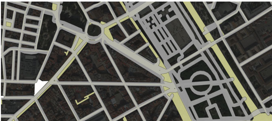
Fig. 4 Polygon-based approach for integrating UA and OSM datasets: grey polygons represent OSM line features buffered by a chosen distance, white polygon represents OSM pedestrian area; green polygon comes from UA dataset of land use type 'Roads and associated land'
