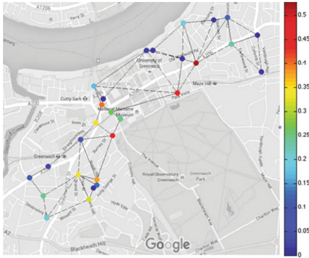
Fig. 10 The betweenness centrality of each node shown with a heat scale ( red indicates the highest centrality value and blue the lowest) considering collective motion with proportionally distributed node resistance
