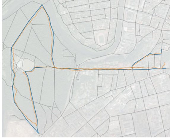
Fig. 7 GPS snapping algorithm: bright line indicates original GPS track; dark line indicates USN edges to which the GPS track has been snapped
