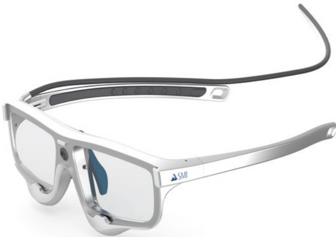
Fig. 6.3 Example of a mobile eye tracking system (reproduced with permission of SensoMotoric Instruments, Teltow, Germany)
