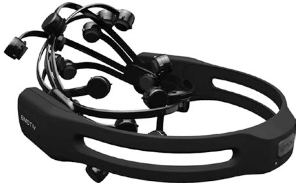
Fig. 6.2 Example of an electroencephalography measurement system (reproduced with permission of Emotiv, San Francisco, CA)
