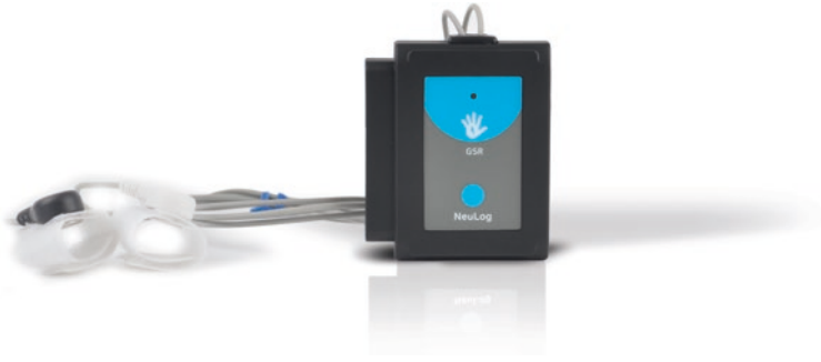
Fig. 6.1 Example of a skin conductance response measurement system (reproduced with permission of NeuLog, Rochester, NY)
