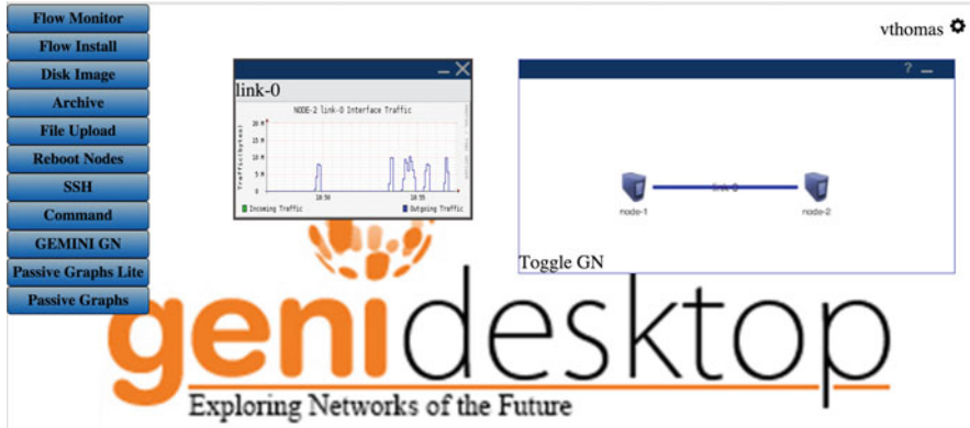
Fig. 14 GENI desktop showing graph of traffic on a network link
