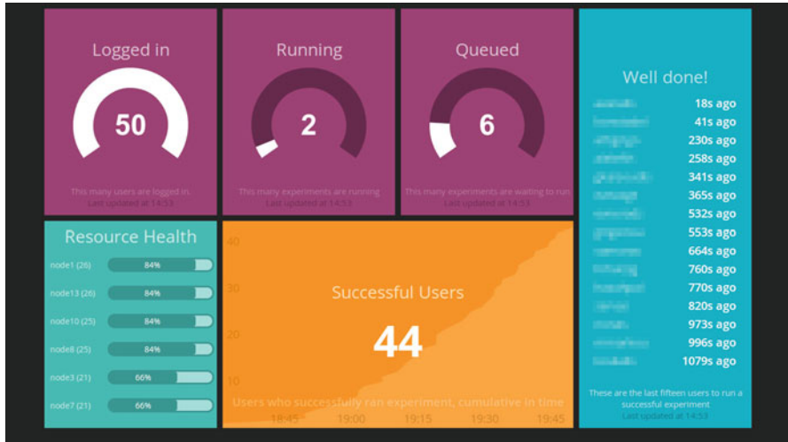
Fig. 3 During a lab session, instructors can see in real time the number of students logged in to the testbed console, the number of experiments currently running, the number of experiments submitted and waiting for available resources to run, the usernames of the students who most recently ran a successful experiment, and the “health” of the testbed resources used in the lab (in terms of the ratio of success of experiments run on each resource)
