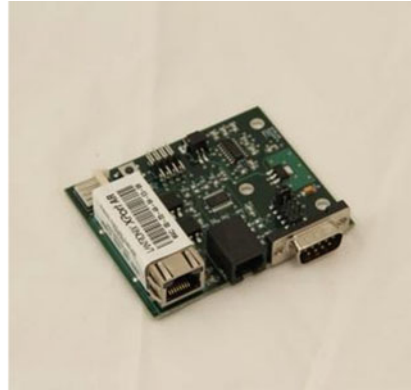
Fig. 9 ORBIT Node Chassis Manager (CM) and photo of the CM board
