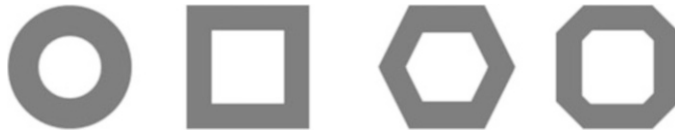
Figure 6.19 CenSurE bilevel center surround filter shape approximations to the Laplacian using binary kernel values of 1 and -1 , which can be efficiently implemented using signed addition rather than multiplication. Note that the circular shape is the desired shape, but the other shapes are easier to compute using integral images, especially the rectangular method
