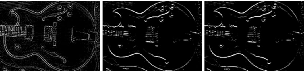
Figure 6.2 Candidate edge interest point filters. (Left to right) Laplacian, derivative filter, and gradient filter
