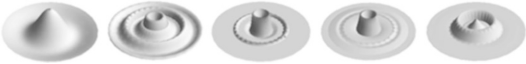
Figure 3.25 Various 2D wavelet shapes: (left to right) Top hat, Shannon, Dabechies, Smylet, Coiflett
