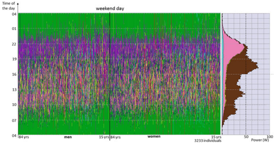
Fig. 11.5 The load profiles of a weekend day from the aggregate activity pattern of a population based on the activity sequences of 3233 individuals. The coloring in the load profiles follows the color of the legend Fig. 11.4 and again the load profile yields the estimated averaged of these activities of the sample ( N = 3233 )
