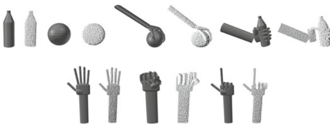
Fig. 5 The 3-D models and their corresponding point clouds generated for our dataset
