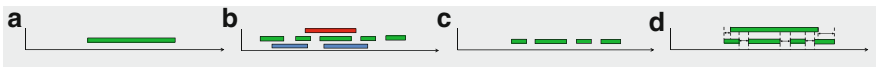
Fig. 12.3 Event matching process. (a) An event of type B in candidate. (b) An example. (c) All events in the example of type B that overlap with the type B event in the candidate. (d) The mismatch (denoted by \leftrightarrow ) calculated by this process
