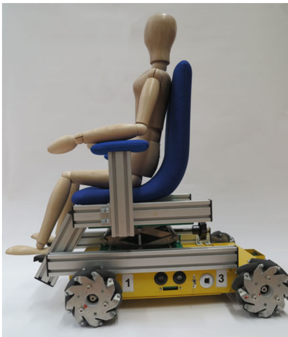
Fig. 3 Mobile robot based on the 4 WD Mecanum wheel mobile kit from NEXUSrobot and controlled by a plugin based software “RobotController”
