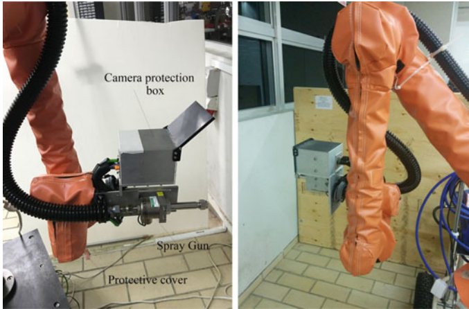
Fig. 2 Manipulator setup outfitted with camera, spray gun and protective covers
