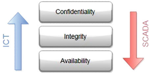
Fig. 1 The comparison of ICT and SCADA cyber security [3]
