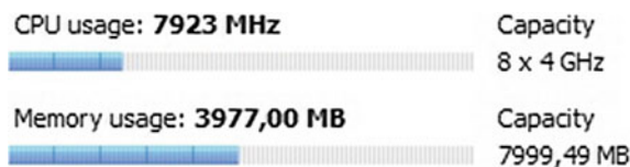
Fig. 1 Utilization of CPU and RAM on the second test computer with installed VMware vSphere 5.1hypervisor when four virtual machines were running
