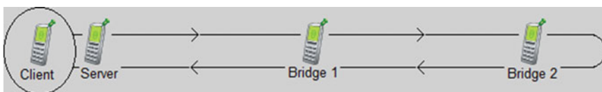
Fig. 1 Layout of the simulation topology. Arrows indicate the motion of the Client node
