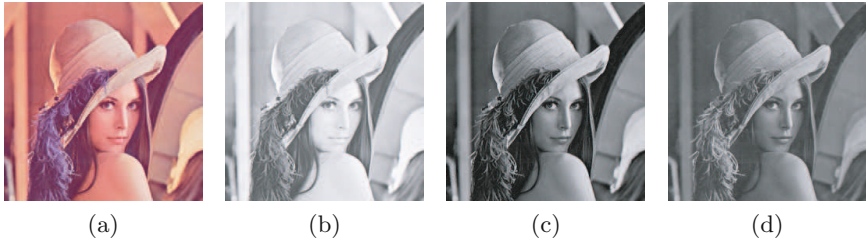
Fig. 2. Original color image and its R, G, B components: (a) Original image, (b) R component of the original image, (c) G component of the original image, (d) B component of the original image.
