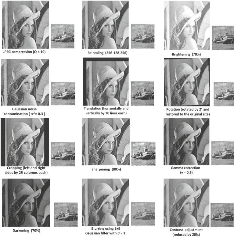
Fig. 5. Watermarked Lena image attacked by different types of attacks and the extracted watermark images.
