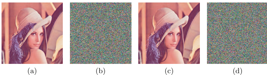
Fig. 5. Key sensitivity analysis in decryption phase: (a) Original image of Lena, (b) Encrypted image with key k_0 , (c) Decrypted image with key k_0 , (d) Decrypted image with key k_1 .
