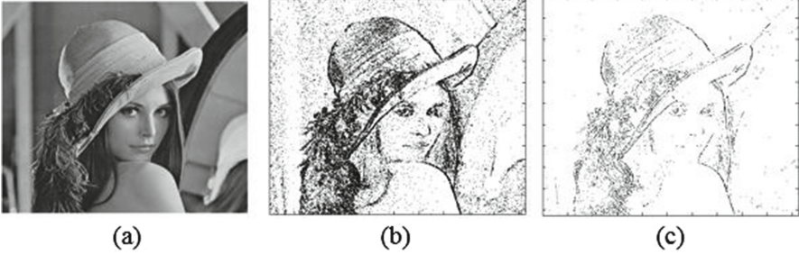
Fig. 2. (a) Lena image. (b) Texture masking JND_T(I_o) with sliding windows 3 \times 3 . (c) Edge masking JND_L(I_o)
