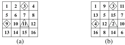
Fig. 7. MSFA pattern: (a) MSFA1, (b) MSFA2. If the interpolation target band of Step 1 is band 1 and t is two, a position surrounded by a triangle is the target pixel in Step a , and a position surrounded by a diamond is the target pixel in Step b .
