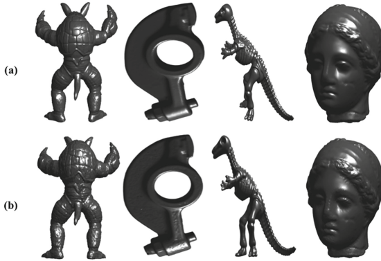
Fig. 3. Some models from the LIRIS/EPFL general-purpose database and their distorted versions: (a) reference meshes. (b) distorted meshes, from left to right are respectively: Armadillo with global noise, Rockerarm with noise in smooth regions, Dinosaur with global smoothing, and Venus with noise in rough regions.
