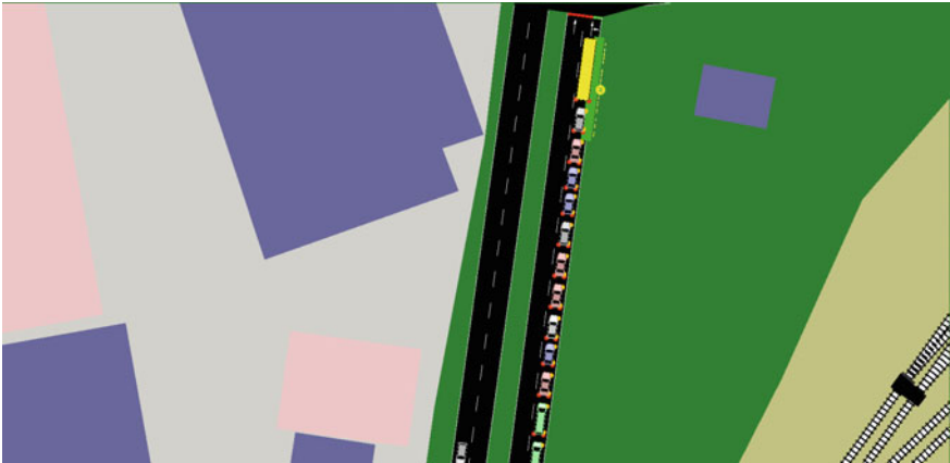
Fig. 5 Eighty people boarding a bus cause the bus to block all right turning vehicles for 40 s, resulting in a congestion on the right lane
