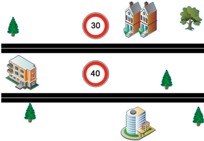
Fig. 4 Urban scenario with speed limits 30 and 40 km/h, two lanes in the same direction
