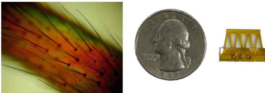
Fig. 1 Setae (left) and hair sensor (right) compared to Quarter (center)
