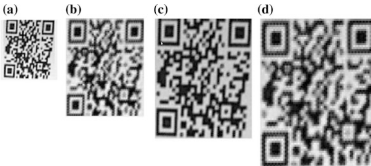
Fig. 6 Image of QR code observed at a distance: a 1.5 m, b 1.0 m, c 0.7 m, d 0.5 m
