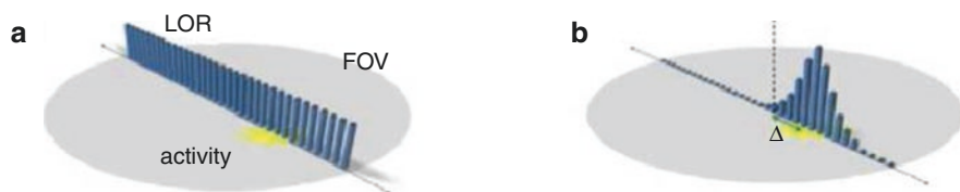
Fig. 13.7 (a) In ordinary PET, the counts in a line of response are assigned with equal probability to all of the pixels along the corresponding line in the image matrix. (b) In time-of-flight PET, the counts can be localized within a limited segment of the line of response. FOV field of view; LOR Line of response (Reproduced with permission of the IAEA from PET/CT Atlas on Quality Control and Image Artefacts; IAEA Human Health Series No. 27; ©IAEA; Published 2014)
