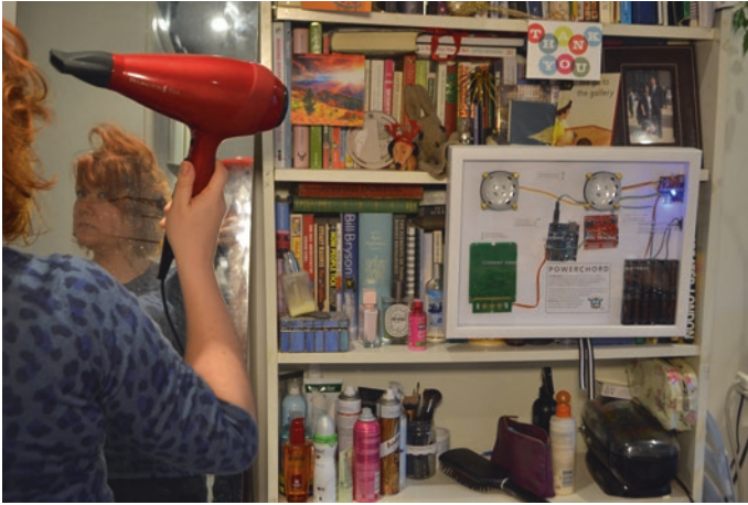
Fig. 23.6 A Powerchord prototype being tested monitoring a hairdryer
