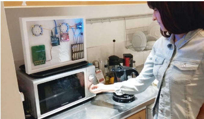
Fig. 23.5 A Powerchord prototype being tested in a kitchen environment, monitoring a microwave oven and an electric kettle
