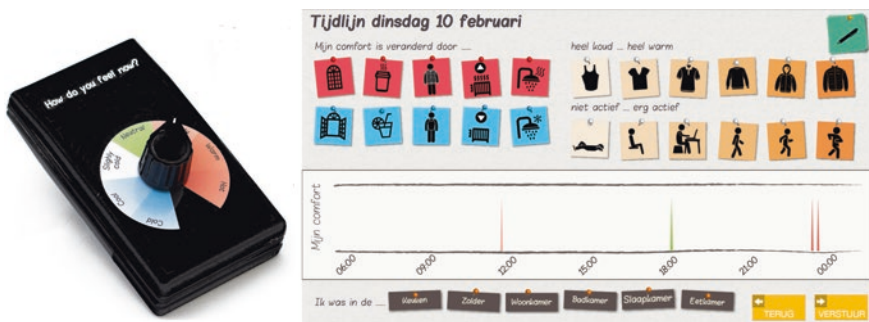
Fig. 12.3 Left—comfort dial; Right—heating practices diary: color coded peaks in the timeline represent inputs from comfort dial, the icons are draggable to indicate heating and cooling practices (top-left of the timeline), level of activity and clothing (top-right of the timeline) and location (bottom of the timeline)
