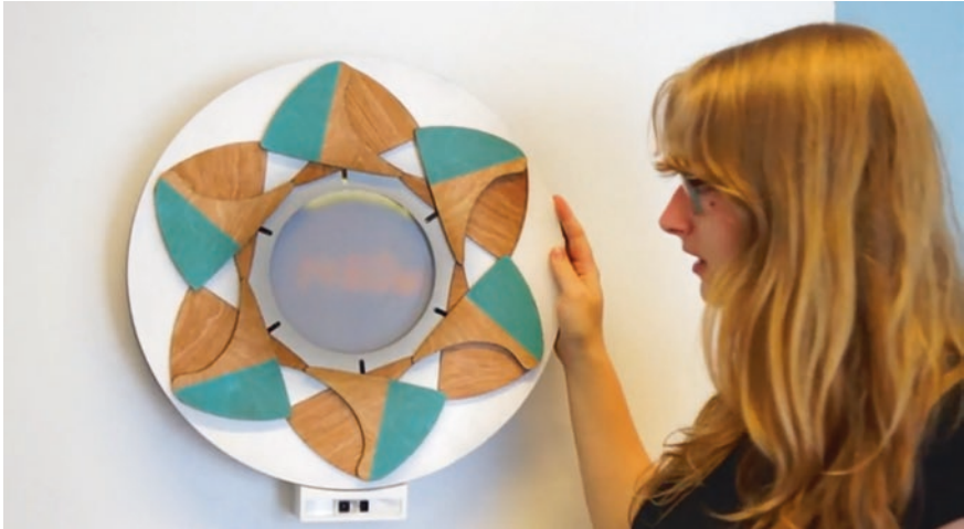
Fig. 25.3 Neo is an aesthetically attractive wall-mounted device that allows office occupants to set an energy goal for the day and provides both ambient, and detailed feedback on current energy consumption at the office
