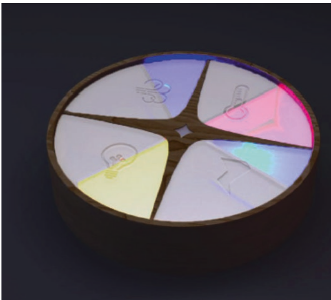
Fig. 22.2 Illustration of an energy feedback display for offices, which shows observed energy usage and average, preferred temperature, light, and perceived air quality
