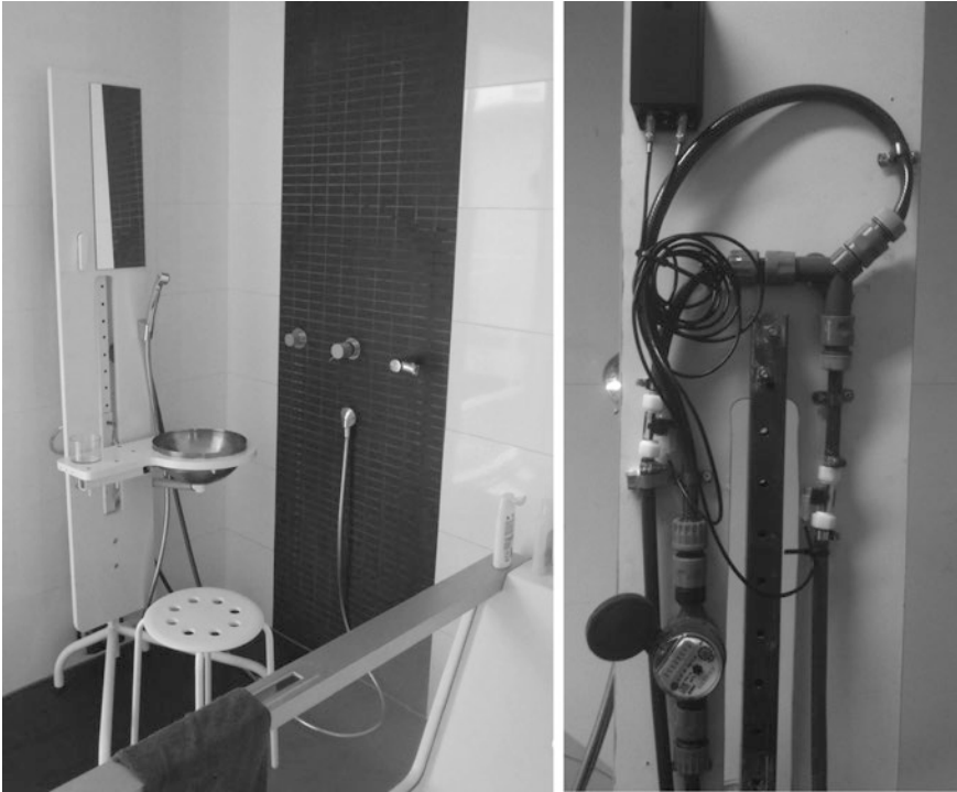
Fig. 6.1 The splash prototype installed in a shower during a field trial ( left ) and the back of the prototype with water meter and logger device ( right )
