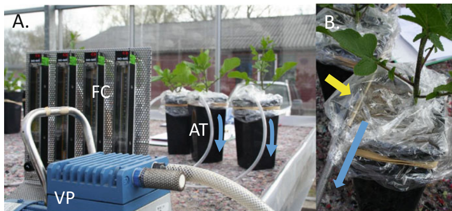
Fig. 8.2 Overview (a) and a detail (b) of a root headspace sampling set-up using direct thermal desorption tubes (indicated in by the yellow arrow in b). The blue arrows indicate the direction of the airflow. Labels: VP vacuum pump, FC flow controllers, AT air tube. The volume of the root headspace is restricted by mounting a pretreated frying bag around the base of the stem. The tubes are inserted into the bags via slit. Air is pulled over the trap via vacuum pump ('pull' system). For more details, see Crespo et al. (2012). Photographs: Nicole M. van Dam
