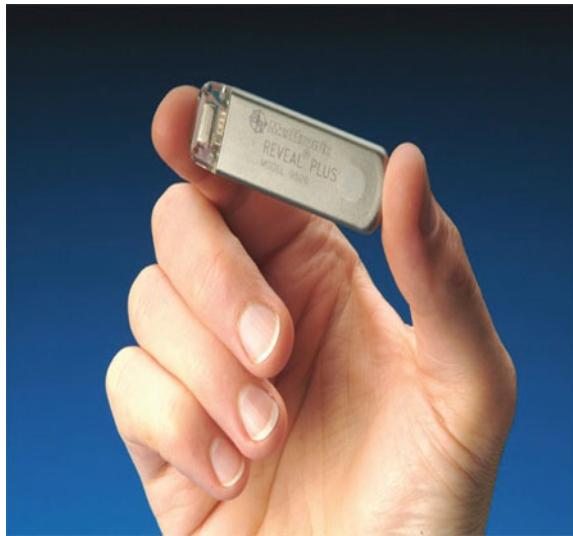
Fig. 5.8 Implantable loop recorder ( Courtesy Medtronic )
