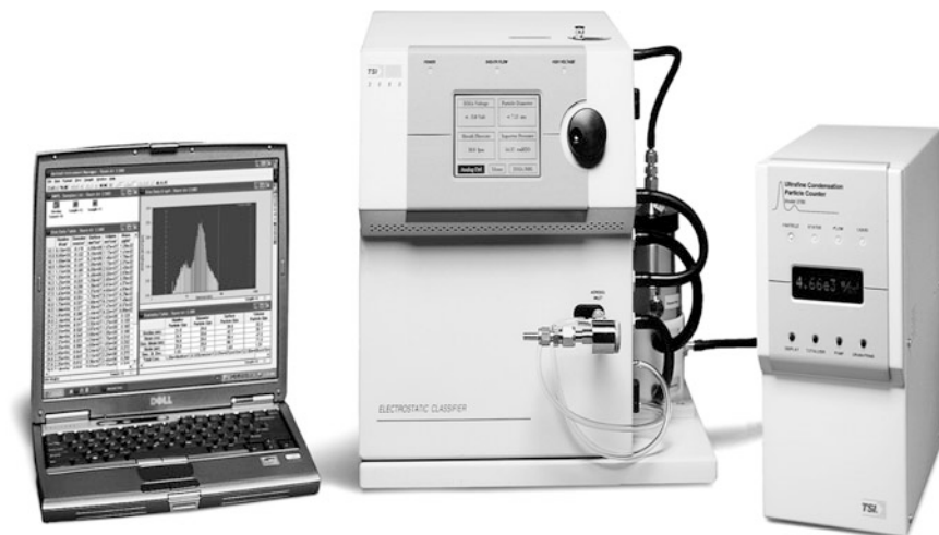
Fig. 10.10 Scanning mobility particle sizer (Permission TSI, Inc.)
