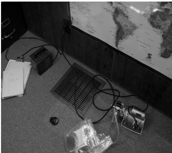
Fig. 10.18 Viable contaminant monitoring apparatus with agar plates
