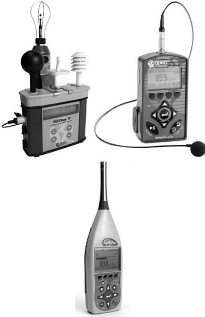
Fig. 10.17 Monitors for heat stress ( left ), noise dosimetry ( center ), and sound level measurement ( Permission Quest Technologies, Inc. )
