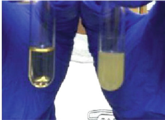
Fig. 16.10 A direct comparison of bacterial growth in samples with ( left tube ) and without ( right tube ) a silver coating. Cloudiness of the liquid in the right tube is indicative of bacterial growth whereas the tube on the left contains a clear amber solution indicating absence of growth [17]
