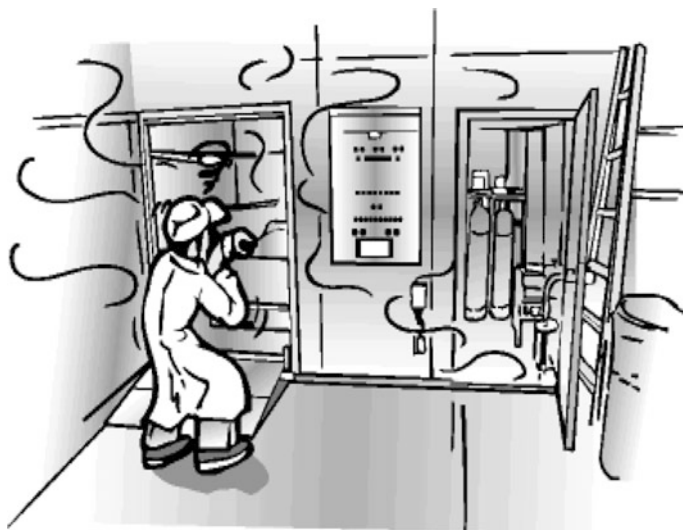
Fig. 10.2 Illustration of ethylene oxide (EtO) leaking from a sterilization chamber ( Permission Japanese Advanced Information Center for Safety and Health )
