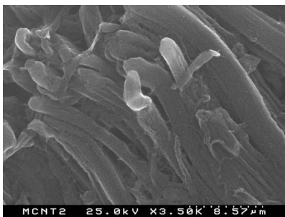
Fig. 12.6 As-grown CNTs in bundle form synthesized using the microwave plasma (MP) CVD method
