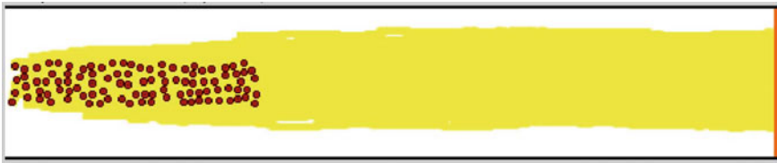
Fig. 4 Evacuation simulation in a corridor with 100 people, showing the influence of the input variable AE on the route choice (yellow) up to the exit
