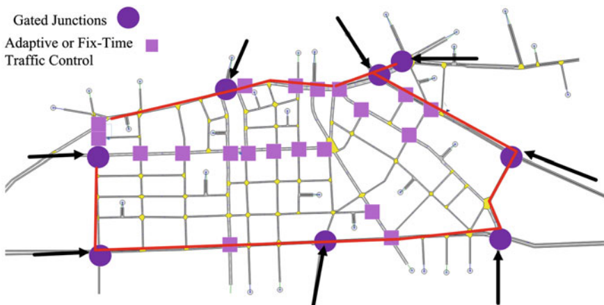
Fig. 1 Part of Chania urban network modelled in AIMSUN; PN is indicated by bold red line
