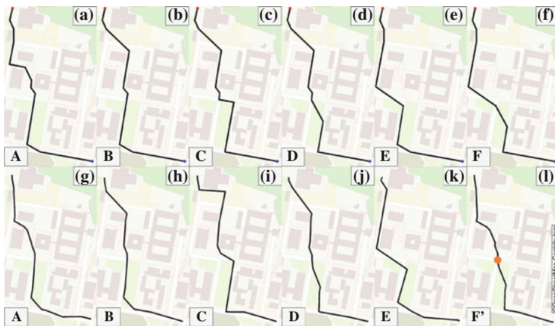
Fig. 3 The measured walking routes of the festival visitors A to F (a–f). The simulation walking routes A to F’ (g–l). The orange marker in (l) indicates the falsely predicted route choice. All routes start at the bottom and end at the top. An extended version of the graph generation method of [9] was used for the case study scenario
