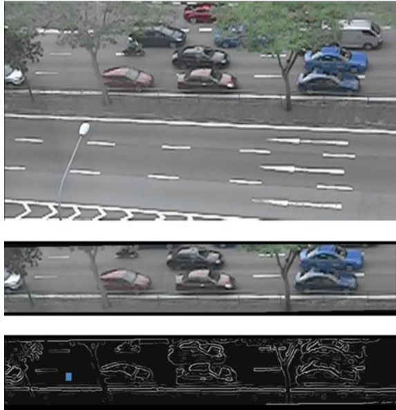
Fig. 1 The top segment part is the complete view of the video; the middle segment is the cropped part where we focus on the fast lane of the traffic from left to right . The bottom segment is the result after conversion of the original video into moving edges using the Canny Edge Detection algorithm
