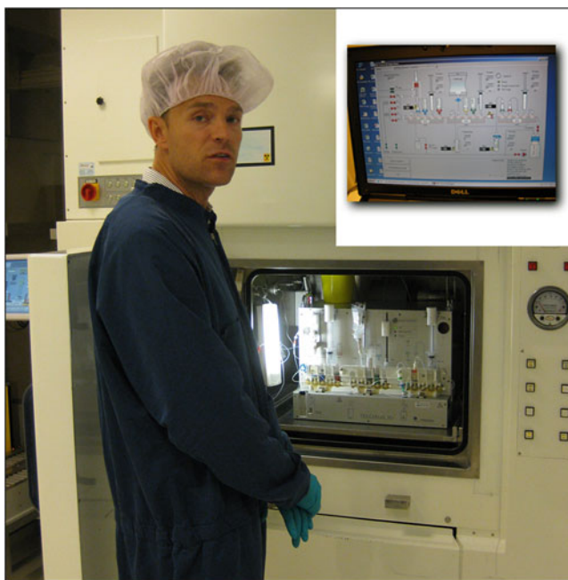
Fig. 6.3 Inside the synthesis lab. Here are the radioactive substances, coming from the cyclotron, synthesised with biological agents in order to make an effective tracer for PET-CT. The insert in the top right corner shows the control software for the process, it is running on a laptop placed on a stool right next to the leaded hot-chamber shown in the main picture
