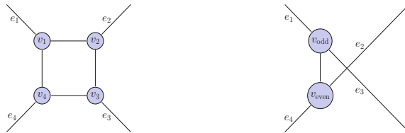
Fig. 1. The 4-cycle on the left is contracted, by identifying v_1, v_3 to a new node v_{\text{odd}} , and identifying v_2, v_4 to a new node v_{\text{even}} , and keeping a single copy of the edge \{v_{\text{odd}}, v_{\text{even}}\} , to obtain the simple cubic bipartite graph on the right.
