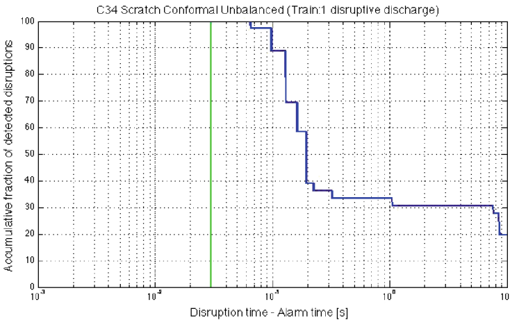
Fig. 3. Results for one-layer CP from scratch on ILW hydrogen campaigns. Green line represents 30 ms before the disruption time. It can be seen that 100% of success rate is achieved with a warning time larger than 30 ms before disruption time (Color figure online).
