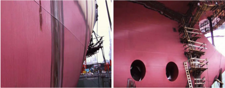
Fig. 1 Manual NDT of weld lines on cargo container ships
