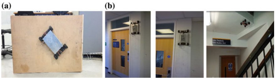
Fig. 17 a The prototype robot turning on the vertical test rig; b Climbing concrete column and ceiling with on board magnetic field sensor
