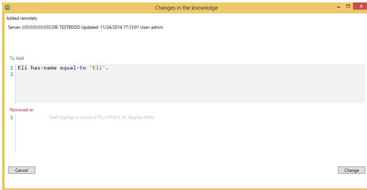
Fig. 3. Screenshot of the window that will be shown to the user when some changes are detected in the current knowledge that the user is editing.
