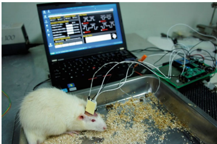
Fig. 10.9 Data collection and electrical stimulation
