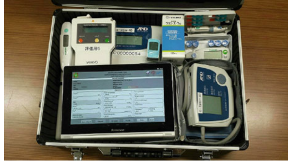
Fig. 18.10 The Portable Health Clinic System package
