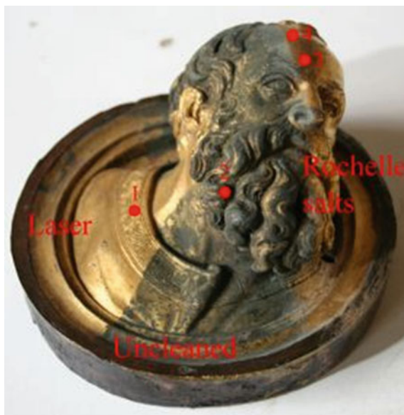
Fig. 1.6 Decorative element (Prophet Head) cleaned by a chemical solution and by laser
