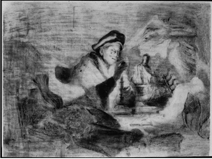
Fig. 3.11 “The Money Changer”, 1st neutron autoradiograph, showing the distribution of manganese. Credits Helmholtz-Zentrum Berlin für Materialien und Energie
