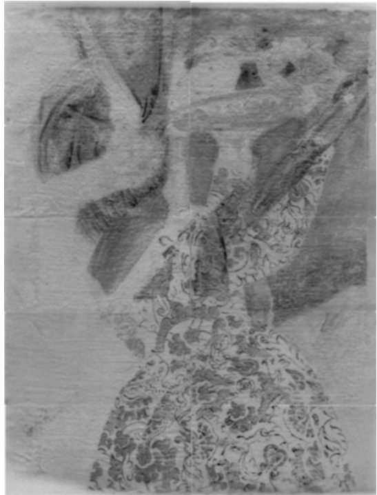
Fig. 3.6 2nd neutron autoradiography, composed of 12 imaging plates, exposure 1 d 7 h to 1 d 11 h after activation. Credits Helmholtz-Zentrum Berlin für Materialien und Energie
