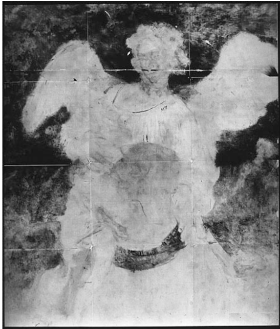
Fig. 3.12 Jacob Wrestling with the Angel, 3rd neutron autoradiograph, showing the arsenic in smalt. Credits Helmholtz-Zentrum Berlin für Materialien und Energie
