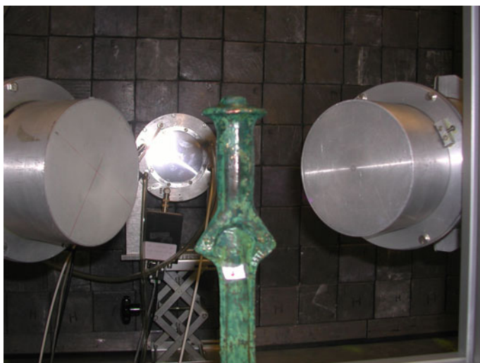
Fig. 12.24 Capture set-up at a 12.5 m measurement station of GELINA. The set-up consists of two \text{C}_6\text{D}_6 detectors and a ^{10}\text{B} loaded ionisation chamber. The sample is a sword with its hilt located in the centre of the beam
