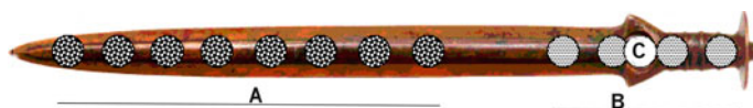
Fig. 12.32 Picture of the Buggenum sword with 13 measurement locations with a beam of 19 mm diameter FWHM. Two series of runs, A and B, at respectively 8 and 4 positions and a run, C, at a fixed position were carried out. The sword is 68 cm long
