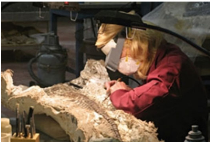
Fig. 7.2 Mechanical preparation—preparator at work fossils are prepared in a laboratory using small, pointed chisels and light-weight hammers. Fine cleaning of important fossils is done under a microscope with dental picks and air scribes (Maropeng 2015c)
