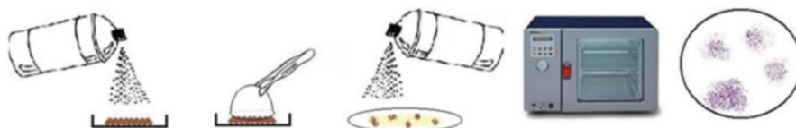
Fig. 15.3 Schematic representation of the new ninhydrin application, where the soil is moisturised using deionised water. A filter paper is than pressed onto the moisturised soil and subsequently sprayed with ninhydrin reagent. The treated filter paper was allowed to dry and then placed for approximately 10 min at 80 °C in an oven, so the result could be interpreted afterwards
