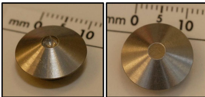
Fig. 7.2 A picture of a DRIFTS sample holder empty ( left ), and containing a soil sample ( right )
