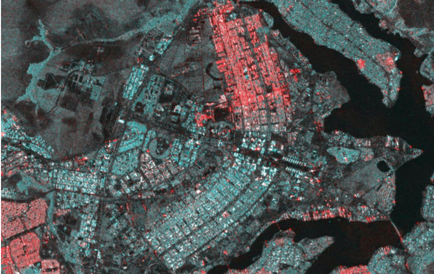
Fig. 9.5 ALOS PALSAR synthetic aperture radar image of the city of Brasilia using bands HH and HV mapped to the R and G/B channels respectively
