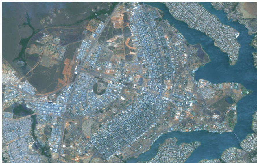
Fig. 9.4 ALOS AVNIR Image of the city of Brasilia using bands 1, 2 and 3 mapped to the B, G and R channels respectively
