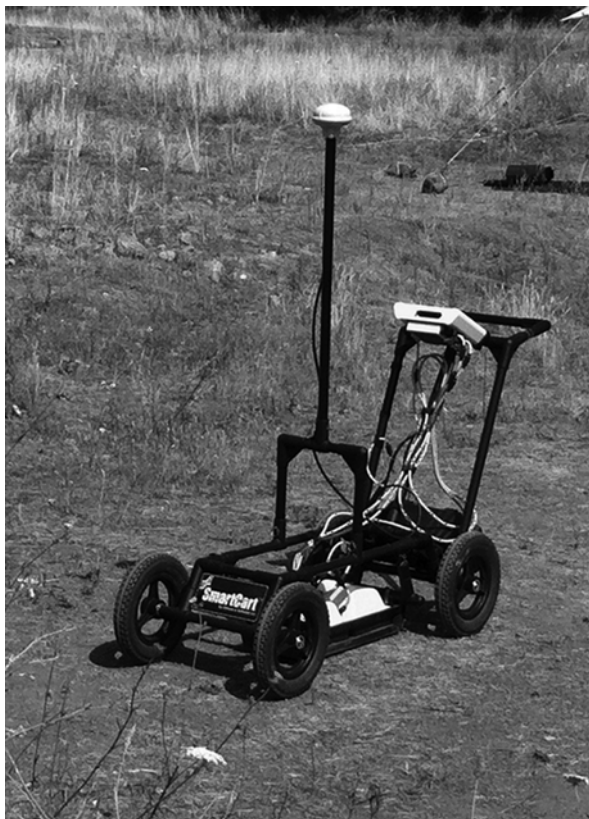
Fig 14.1 A typical GPR system during a forensic investigation: the main transducer unit mounted on a cart, a DVL, and equipped with a GPS
